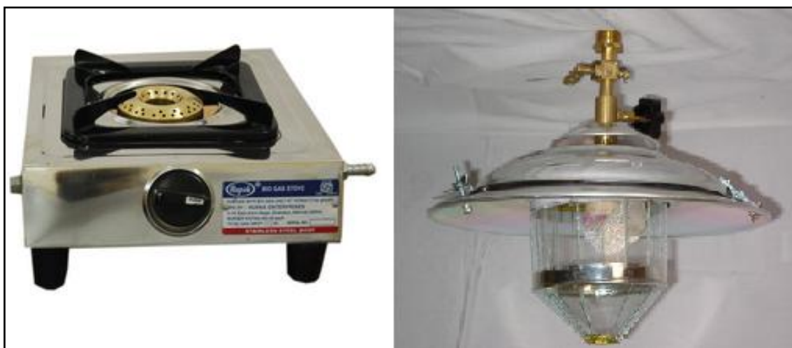
Figure 2-14. Single burner biogas stove (left) and biogas lamp (right). Both are made by Indian company Rupak Enterprises (tradeindia.com, 2010). A LPG burner can be modified for biogas by enlarging the nozzle holes to compensate for the lower pressure.
