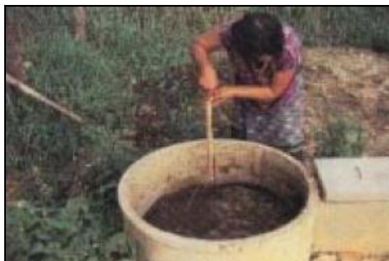
Figure 2-13. The photo shows a woman mixing waste and water for her biogas plant. Notice that the mixing tank is uncovered and she is not wearing any protective clothing (Koottatep, Ompont and Hwa, 2002: 95).
